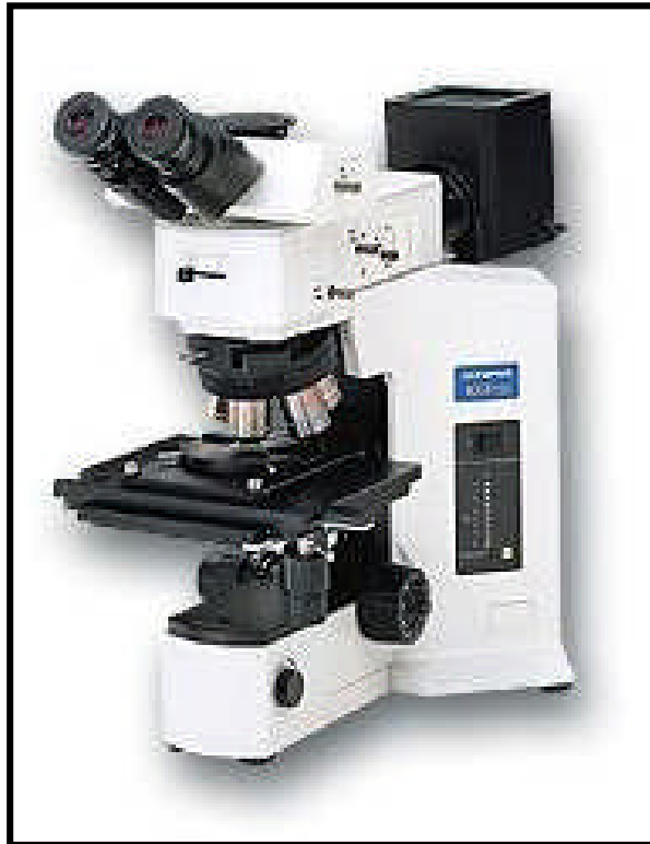
Figure II.3. Microscope optique de type OLYMPUS BX51M.
