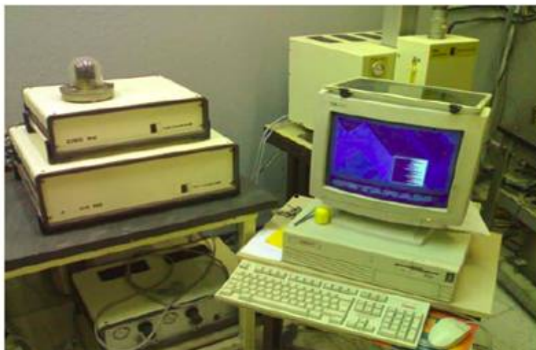
Figure IV.3 Appareil de DSC type SETARAM DSC92.
