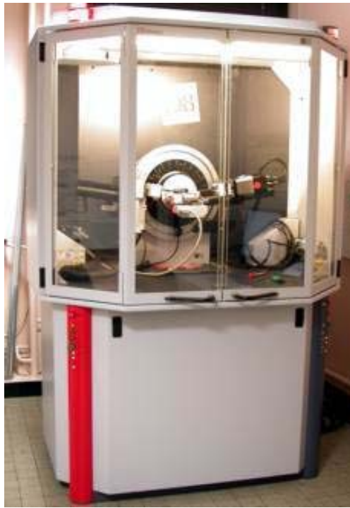
Figure. II.2. diffractomètre de marque BRUKER - AXS type D8.
