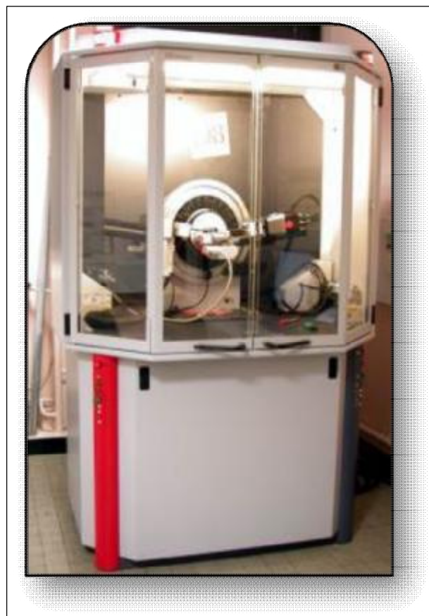
Figure III-1: Image d'un diffractomètre Bruker D8 Advance.
