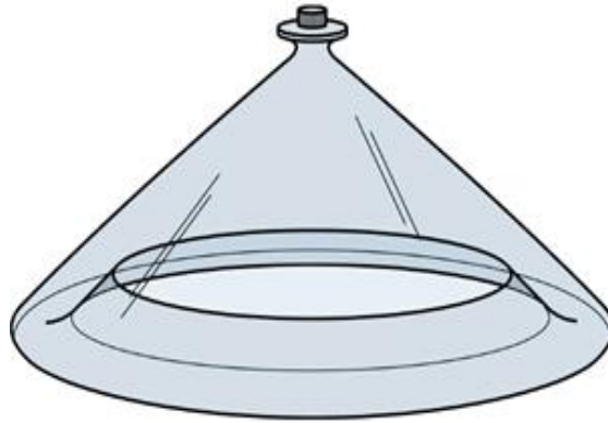
Figure II.17- Distillateur de type watercone
