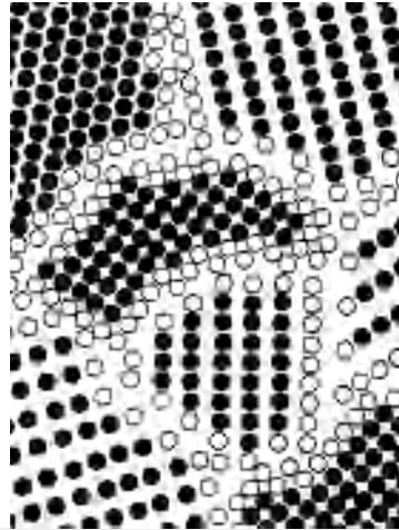
Figure. 2.20: Schematic arrangement of atoms in an equiaxed nanocrystalline metal.
