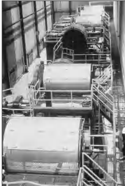
Figure. 2.25: Commercial production-size ball mills used for mechanical alloying. Courtesy of Inco Alloys International.
