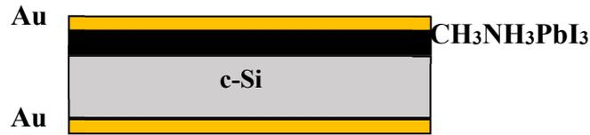
Fig. 1: Schematic drawn of the heterojunction  $\text{CH}_3\text{NH}_3\text{PbI}_3/(\text{P})\text{c-Si}$ .
