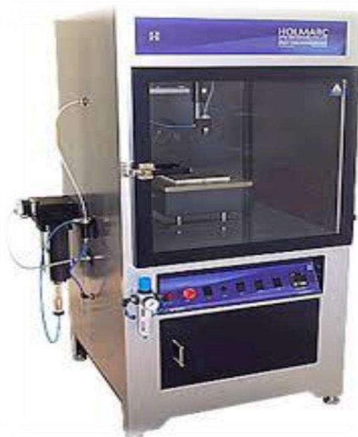
Figure II.4: The deposition system of ultrasonic spray pyrolysis (Holmarc)
