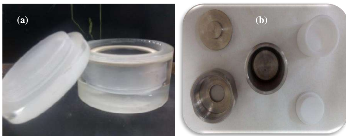
Figure II.10: Autoclave used for preparation of ZnO Nanostructured; (a) polymer and (b) Teflon Lined Sealed Stainless Steel
