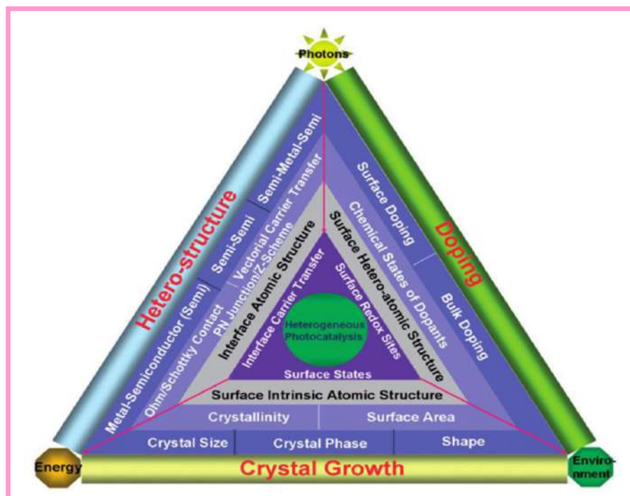
Figure I.7: The relation between crystal growth, doping and heterostructure in semiconductor photocatalysis [51]
