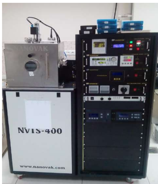
Figure II.8: RF sputtering deposition system of ZnO thin film with different thickness
