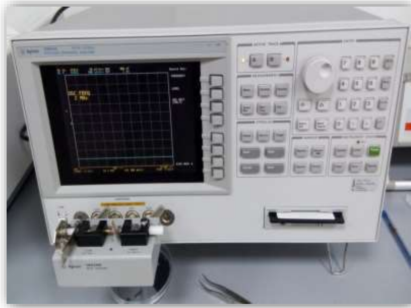
Figure IV.27: The C-V characterization device
