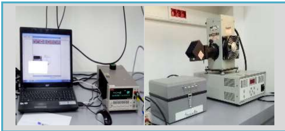
Figure IV.17: I-V measurement system in the dark
