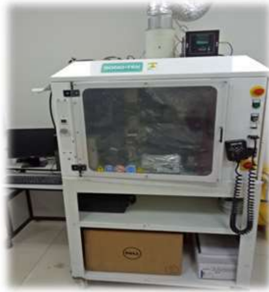
Figure II.15: The deposition system SONO-TEK ultrasonic spray pyrolysis
