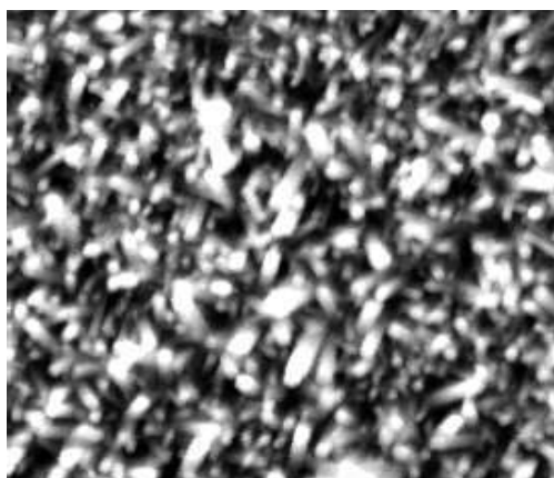
Figure III.37: Typical Micrographs of ZnO Nanorods by hydrothermal at 120°C for 3 h.
