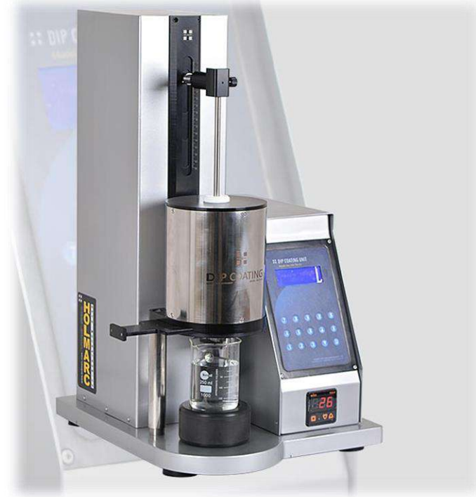
Figure II.6: Deposition system of sol-gel dip coating
