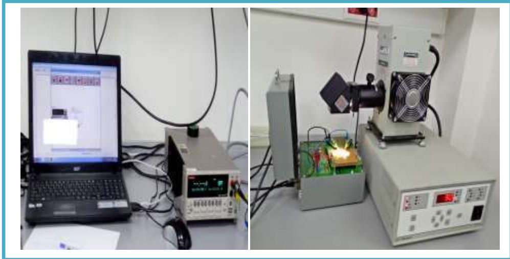
Figure IV.18: I-V measurement system under illumination
