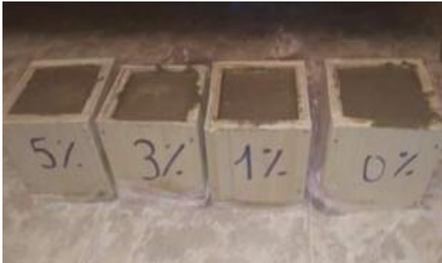
Figure 3.6: Moules cubiques de volume (10 \times 10 \times 10) \text{ cm}^3 .
