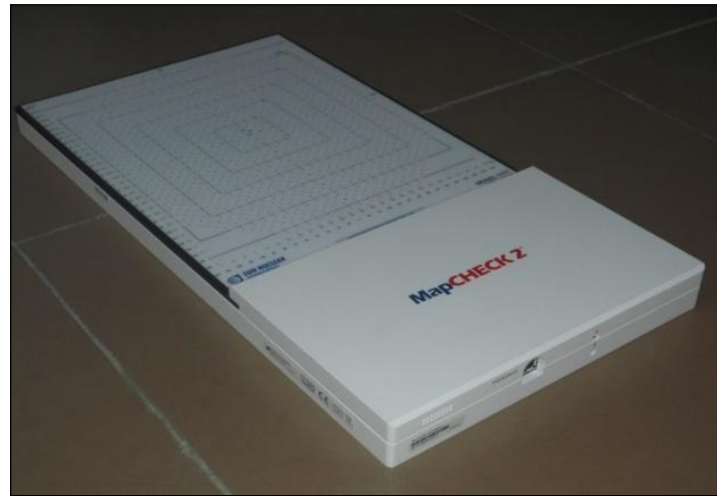
Figure III.5 La matrice MapCheck2. Centre-Anti Cancer ATHENA.
