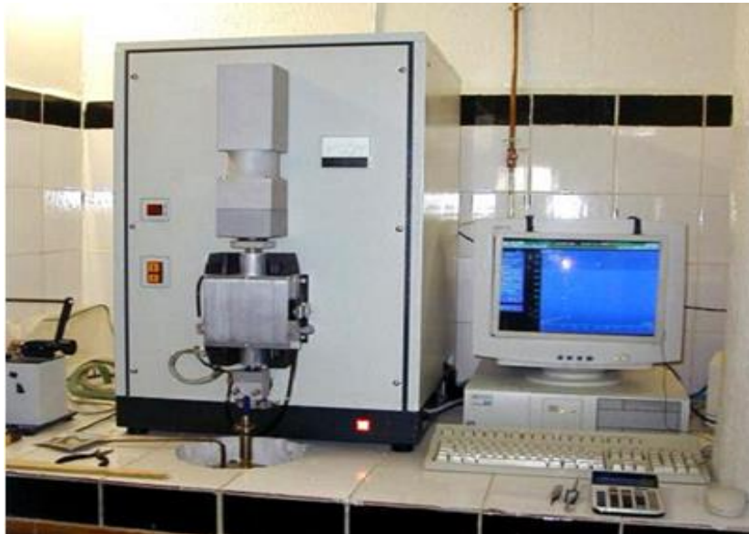
Fig.3.4. The used dilatometer ADAMEL LHOMERGY of DT1000 type, connected to a computer (UC1).
