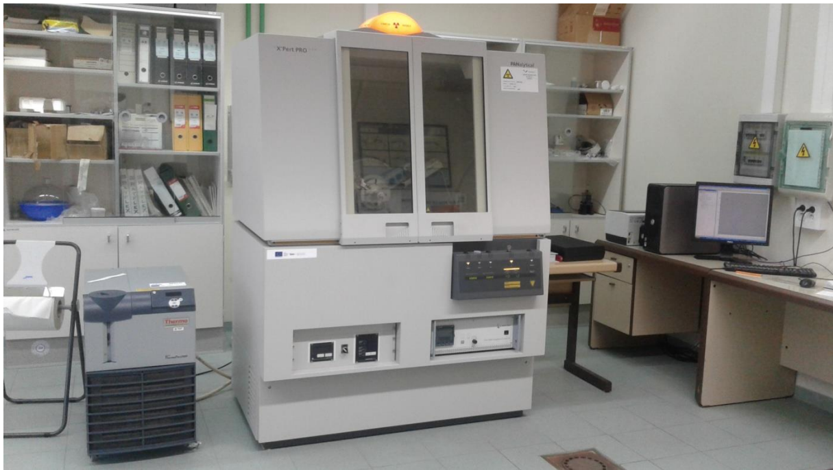
Fig.3.8. The used XPERT PRO Diffractometer (UNIOVI).
