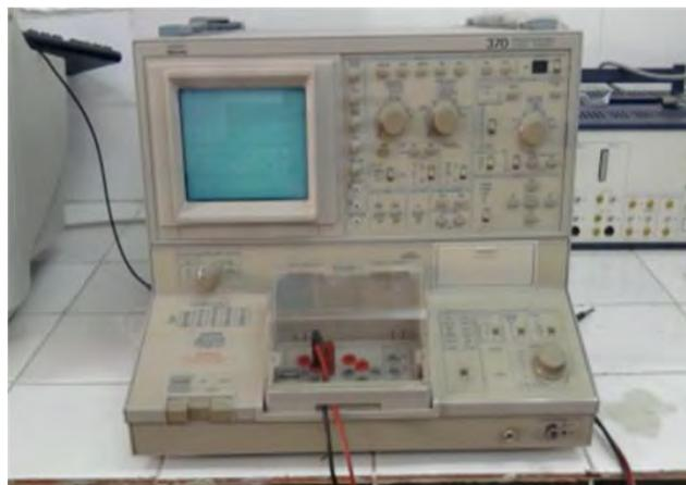
Fig.III.21: Banc de test de la cellule Cu<sub>x</sub>S/CdS (Labo. LCMI, Univ. Constantine 1).
