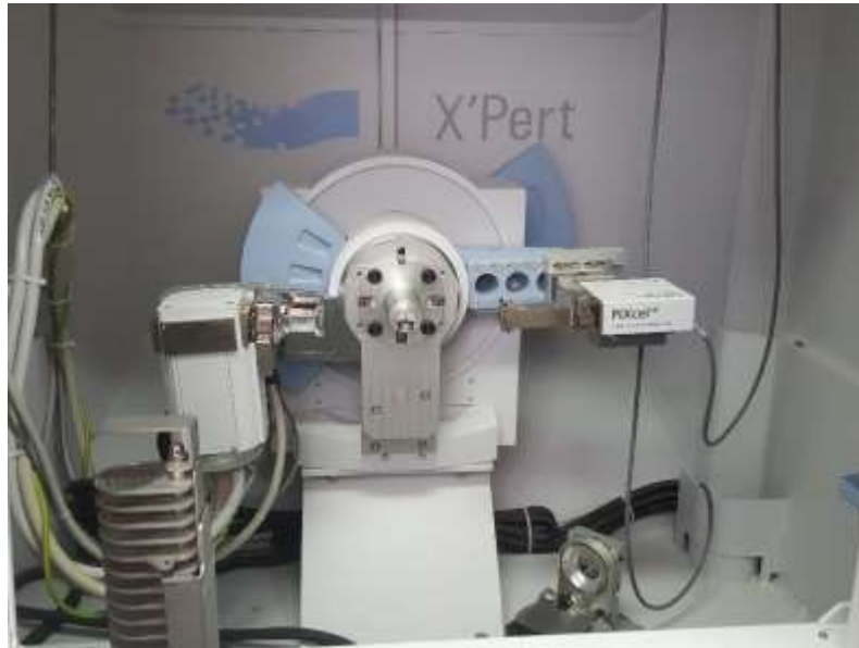
Figure 31: Diffractomètre DRX X'Pert PANALYTICAL.
