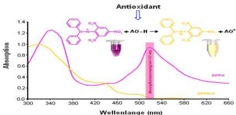
Figure V.1. Structure of DPPH • radical and its reduction by an antioxidant (AO-H). (Adapted from [19]).
