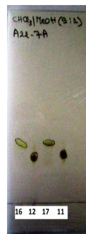
Figure III.5. TLC of separated compounds 16 , 12 , 17 and 11
