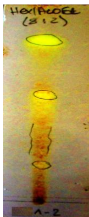
Figure III.10. TLC of subfraction (1+2) from fraction 9 eluted with (CHCl 3 / MeOH, 90:10, v/v) by treating with a Ce(SO 4 ) 2 / H 2 SO 4 .
