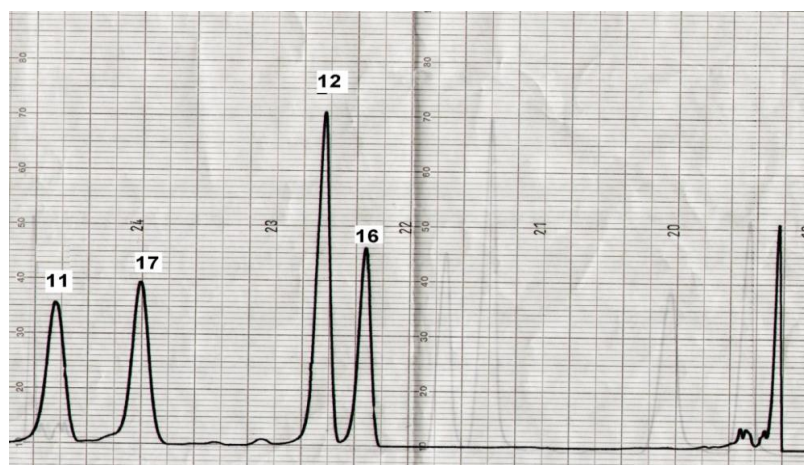
Figure III.4. RP- HPLC Separation chromatogram of fraction (22+23) with acetonitrile / \text{H}_2\text{O} (50:50, v/v).
