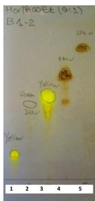
Figure III.8. TLC of Fraction 15 eluted with (Hexane / EtOAc, 90:10, v/v) by treating with a \text{Ce}(\text{SO}_4)_2 / \text{H}_2\text{SO}_4 .
