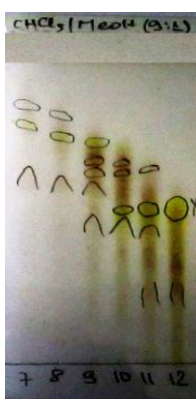
Figure III.9. TLC of Fraction 9 eluted with ( \text{CHCl}_3 / MeOH, 90:10, v/v) by treating with a \text{Ce}(\text{SO}_4)_2 / \text{H}_2\text{SO}_4 .
