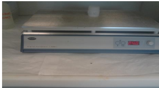
Figure 21. La plaque chauffante (Stuart SD 500)
