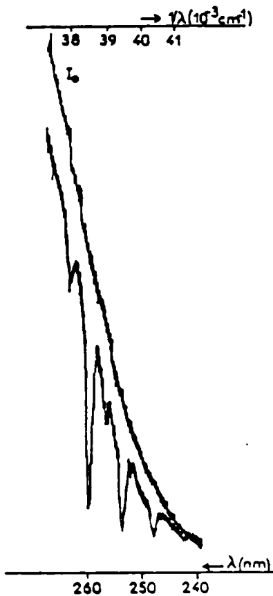
FIG. 2. Absorption spectrum of benzene in nitrogen matrix.
