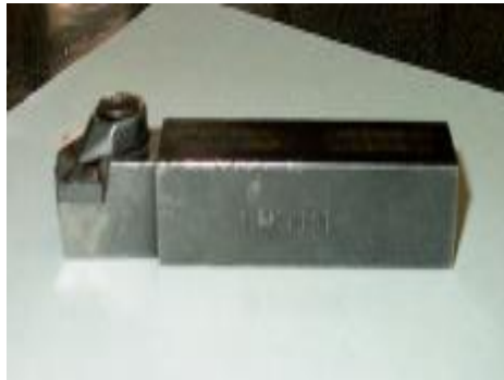
Figure III.1 : Porte plaquette CTGPL 16 16 K16 .
