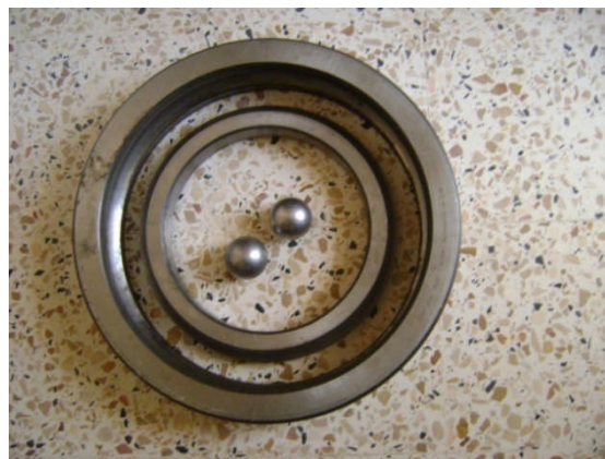
Figure IV.9. Image roulement SKF QJ 1244 N2MA.
