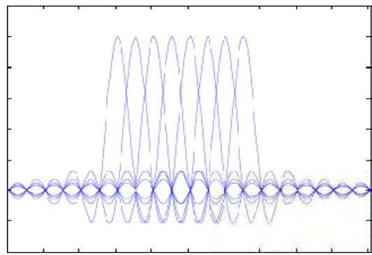
Fig.4.2 Répartition adjacente des spectres
