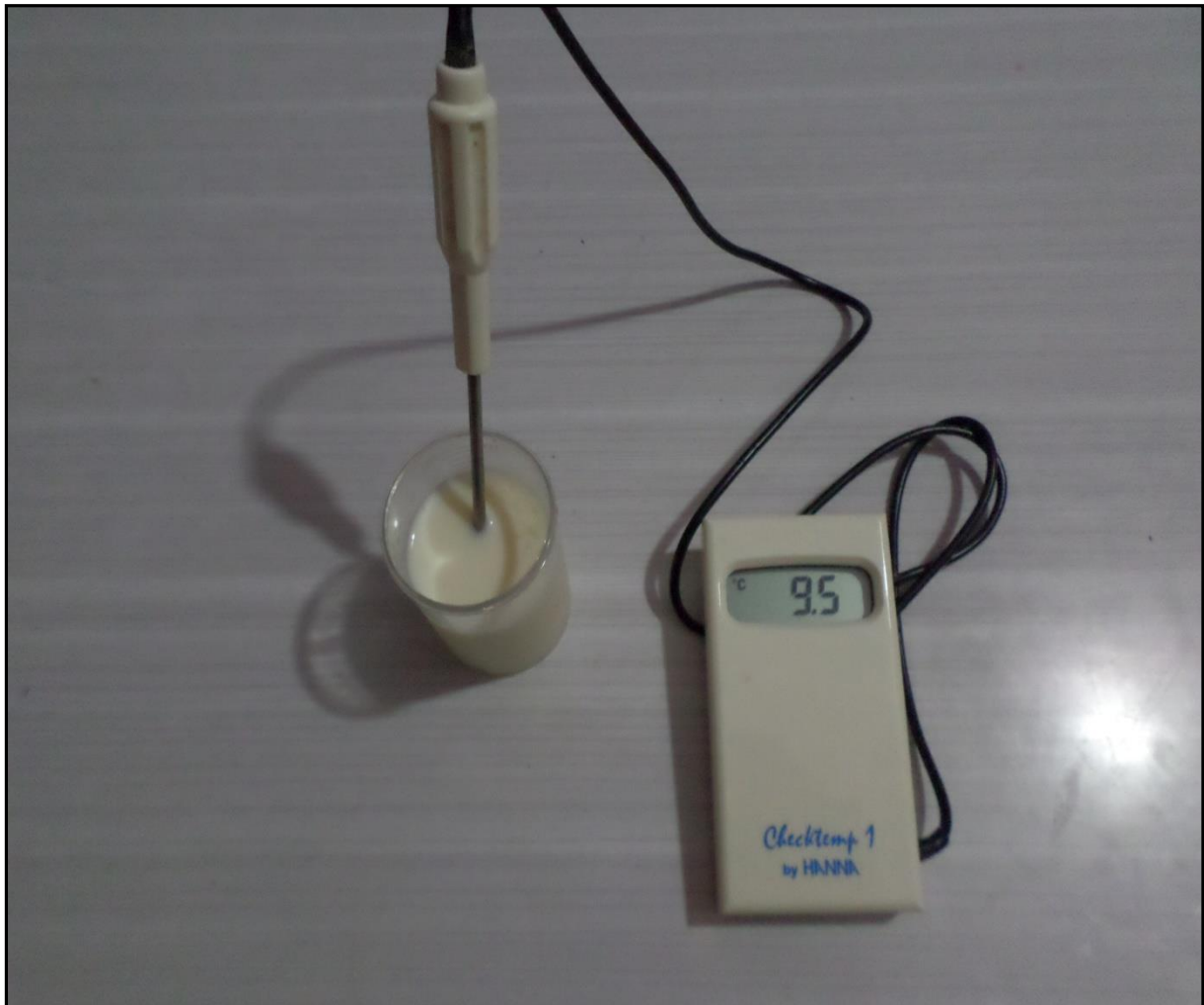
Figure 5: Thermomètre type Hanna Instrument, model HI98509.
