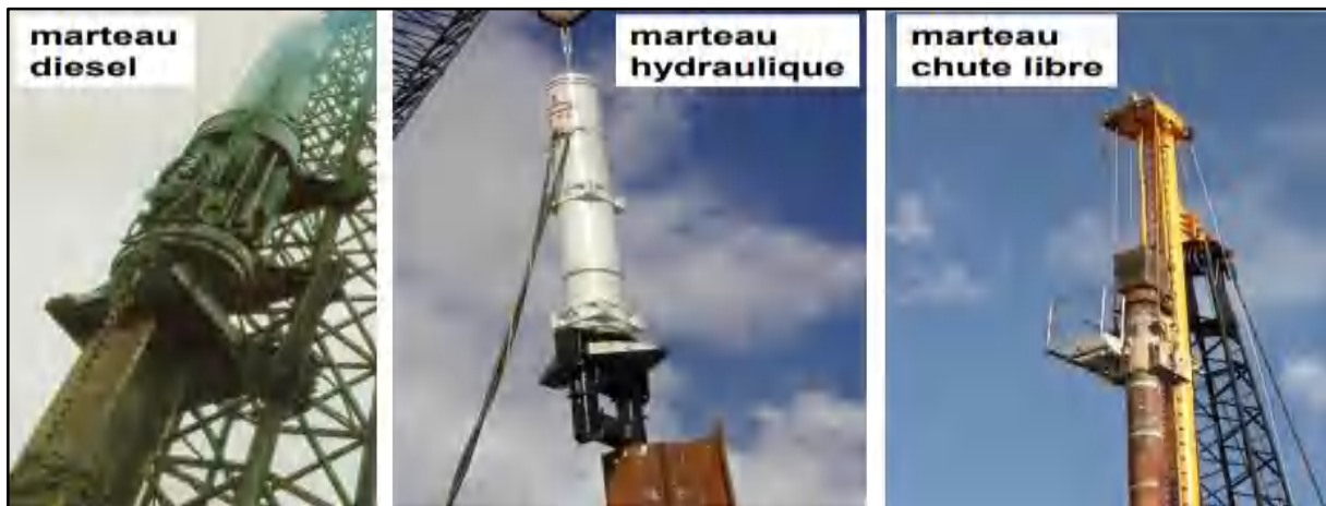
Figure II.9 Outils de battage Pieux/H/palplanches battus [Classe : 4/5/6/7] [8]
