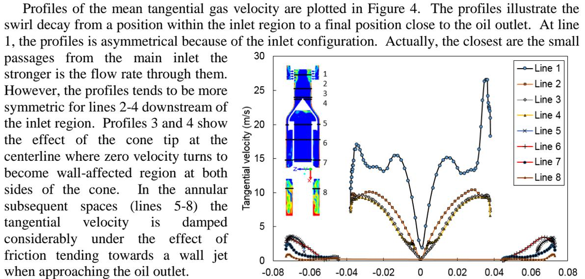
FIGURE 4. Mean gas tangential velocity at different axial positions
