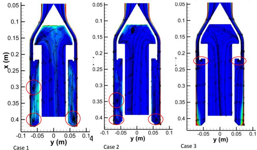
FIGURE 3. Streamtraces superimposed on oil volume fraction within the cone region
